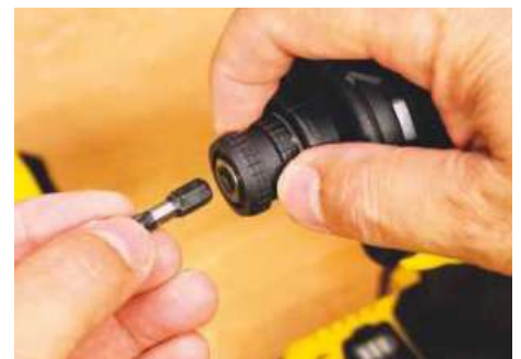
▲ 25mm bits can be used in the impact driver but aren't locked in the chuck
